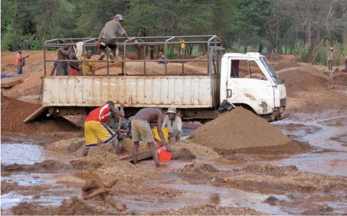
Figure DD-11. Gem-bearing material is shoveled out of the truck and placed in a sieve for washing. Photo © V. Pardieu/GGL.
