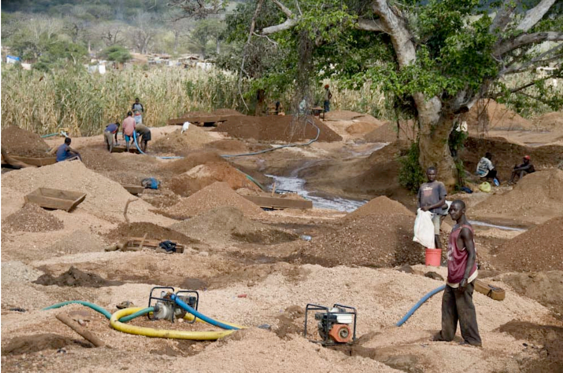
Figure DD-9. Portable pumps were brought to Winza by enterprising individuals to supply water for the washing operations. Photo © B. M. Laurs/GIA.
