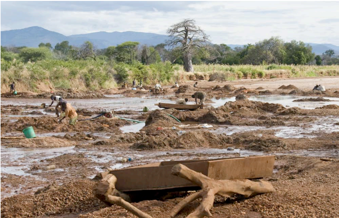
Figure DD-5. Water from the Mtindiri River is used to wash corundum-bearing material. Photo © B. M. Laurs/GIA.
