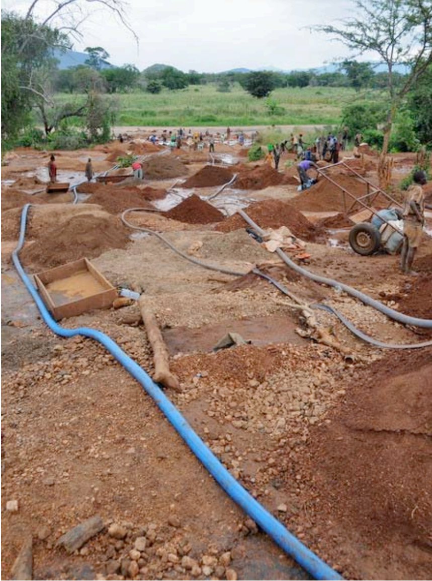
Figure DD-6. At the Mtindiri River, miners use pumps, hoses, and sieves to wash gem-rich material. Photo © V. Pardieu/GGL.
