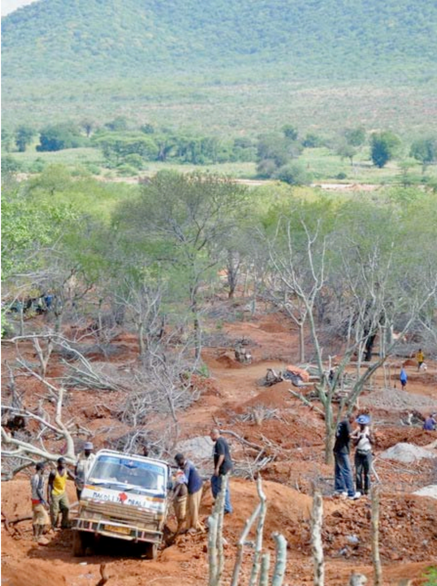
Figure DD-8. A truck is loaded with gem-bearing ground for transport to the nearby river for washing. Photo © V. Pardieu/GGL.
