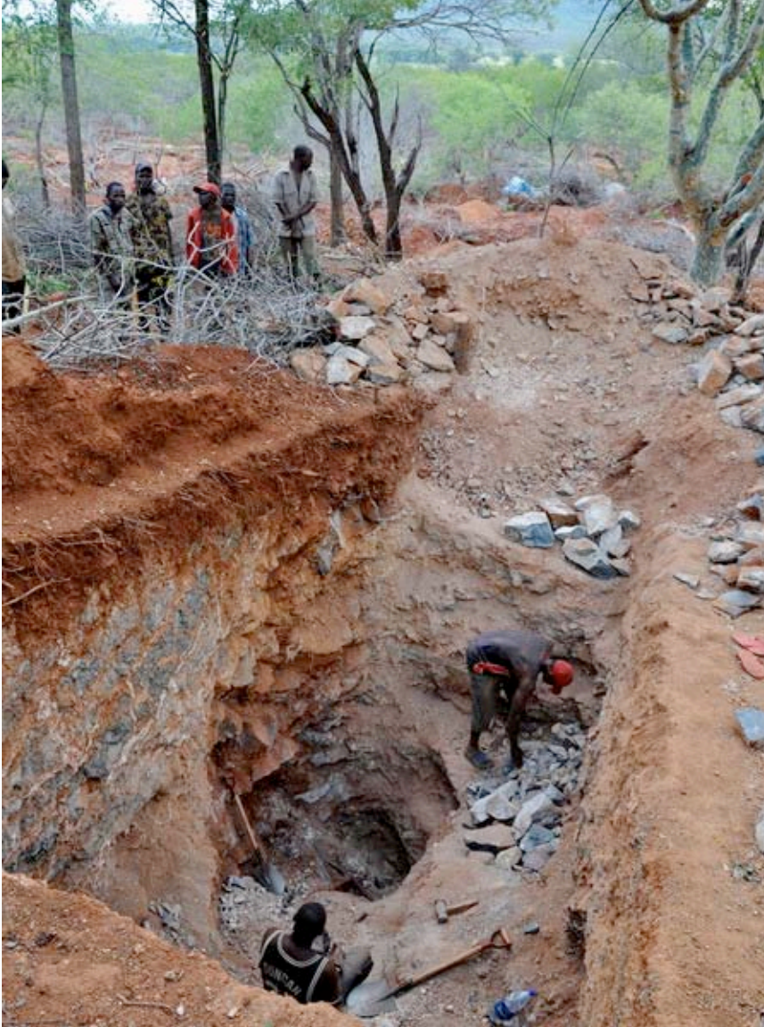
Figure DD-13. Miners have dug through the gem-bearing rust-brown eluvial soil and are recovering sapphires from the underlying hard-rock deposit (amphibolite). Photo © V. Pardieu/GGL.
