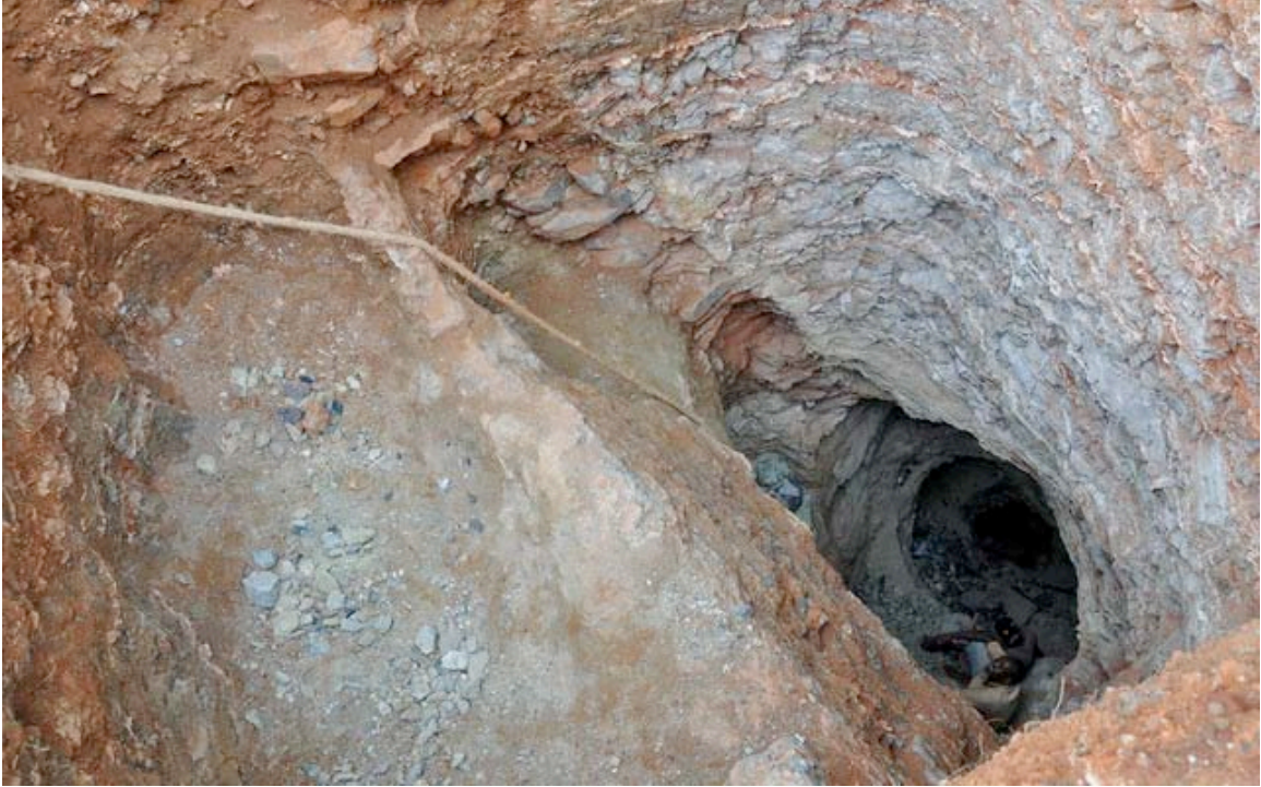
Figure DD-19. Mining pit following an amphibolite vein. Photo © V. Pardieu/GGL.
