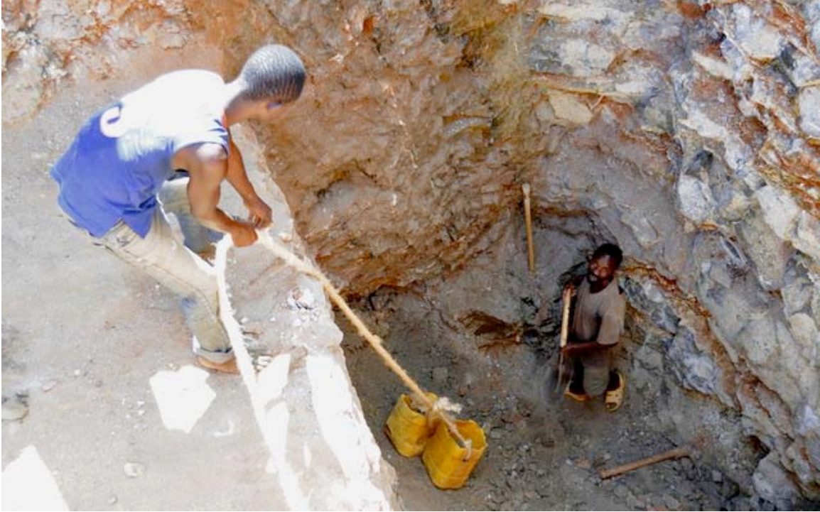
Figure DD-16. A miner removes material from a trench following an amphibolite vein. Photo © V. Pardieu/GGL.
