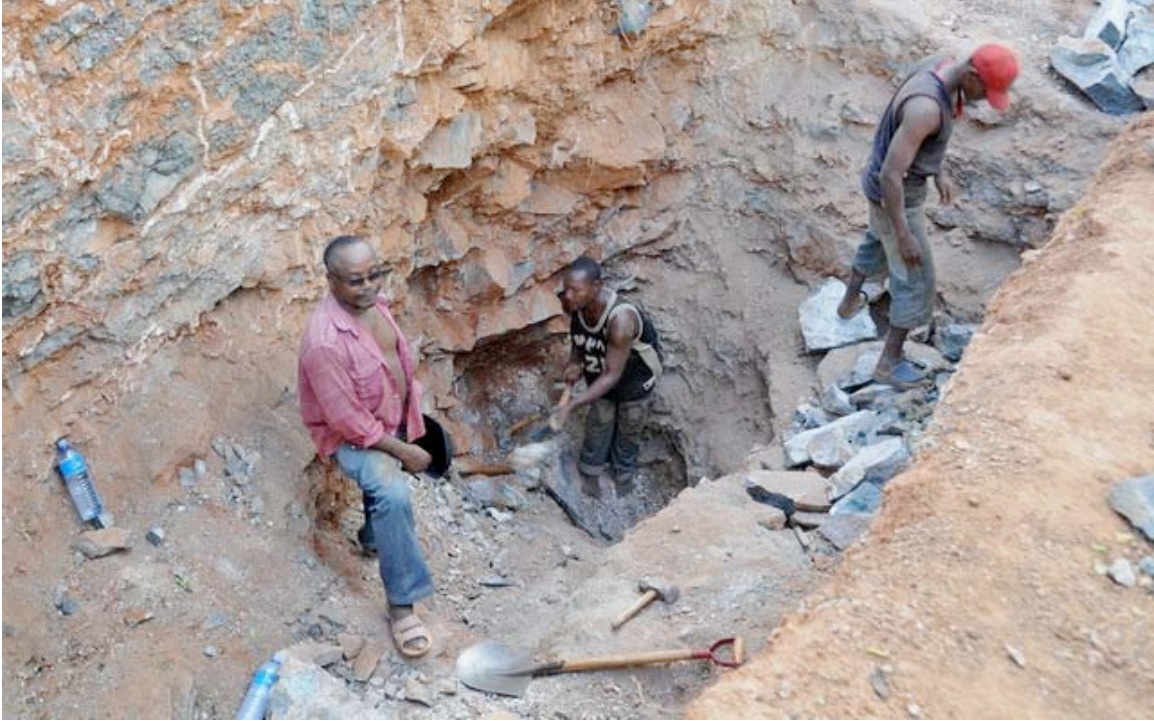
Figure DD-14. Miners follow an amphibolite vein at this hard-rock deposit. Photo © V. Pardieu/GGL.
