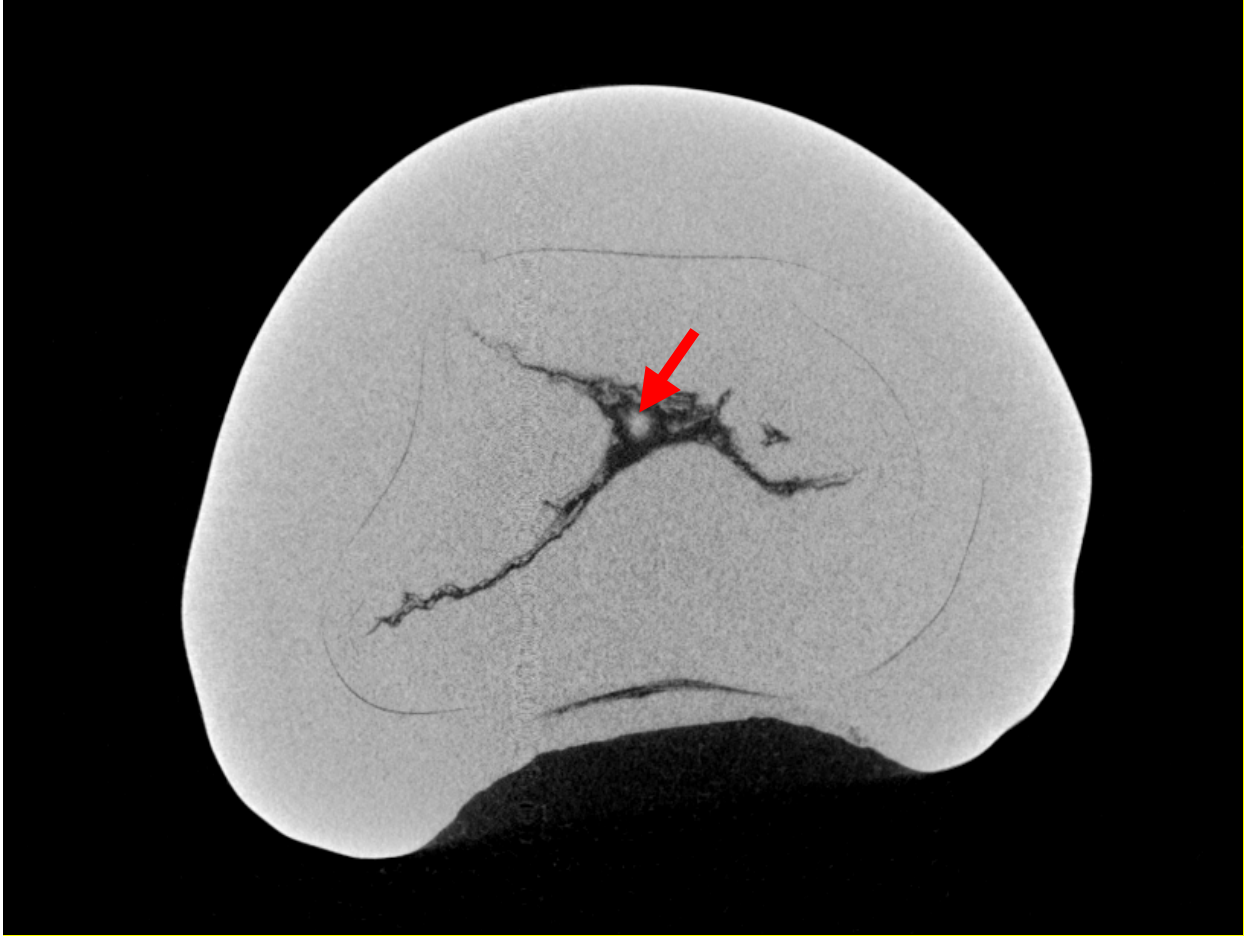
Figure 3. A magnified \mu -CT slice from the Y-direction of pearl 3 (table 3) showing a white seed-like structure in the central irregular void feature (see red arrow).
