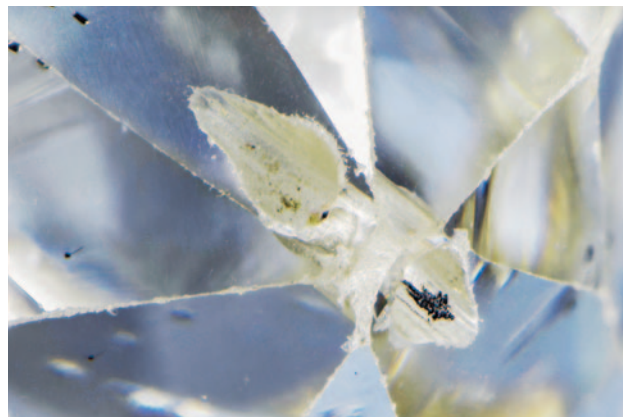
Figure 33. The drill hole at the tip of the stone. Note the unique surface, a remnant of the process of drawing a wire coated with diamond dust and oil back and forth. Photomicrograph by Nathan Renfro; field of view 4.02 mm.
