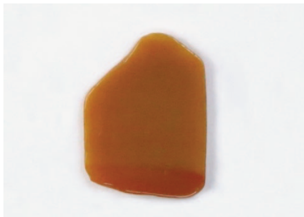
Figure 39. The untreated brownish yellow rough stone, approximately 17.0 \times 22.0 \times 1.5 mm, loaned by the client for analysis. Photo by Xiaoping Shi.
