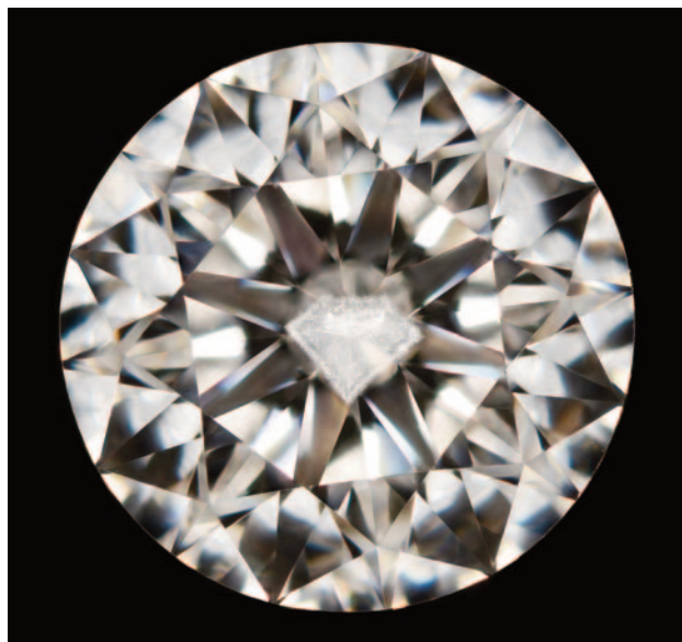
Figure 4. The D-color, 0.53 ct round brilliant diamond has SI 2 clarity due to a distinctive cloud inclusion under the table facet. Photo by Marco Martinez.
