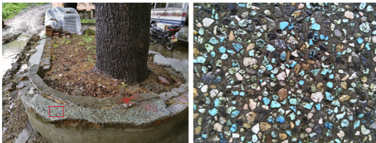
Figure 2. Turquoise fragments (0.2 × 0.2 cm to 1.0 × 1.3 cm) were used as outdoor decorative materials in the 1980s in Yun County, Hubei Province. Photos by Ling Liu.
