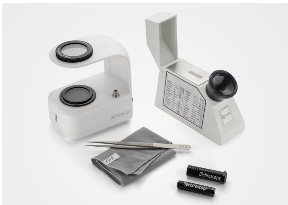
Figure 6. Clockwise from top left: A polariscope, refractometer, dichroscope, and spectroscope are shown with a gem cloth and tweezers. Photo by Emily Lane.
