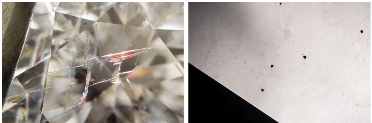
Figure 4. Examples of treatments documented in diamond. Left: Fracture filling in a feather on the table of a laboratory-grown diamond. Right: Reflective lighting displaying numerous laser drill holes in the table of a diamond. Photomicrographs by Nicole Ahline; fields of view 3.57 mm (left) and 4.79 mm (right).
