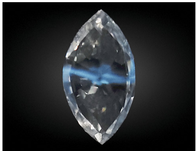
Figure 21. Short-wave UV imaging of the multilayered laboratory-grown diamond showed the thin layer phosphorescing while the rest of the diamond remained inert. Image by Guy Borenstein.
