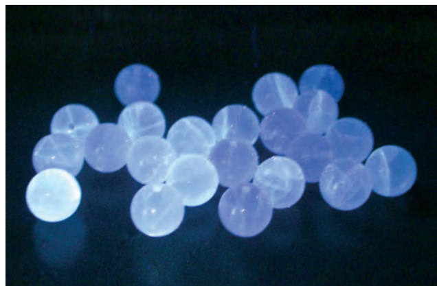
Figure 2. Most of the moonstones fluoresced moderate to strong blue-white to long-wave UV, with the fluorescence visible in the fissures (left). Under short-wave UV (right), most of them either fluoresced weak bluish white (seen in the fissures) or were inert. Photo by Jianjun Li.
