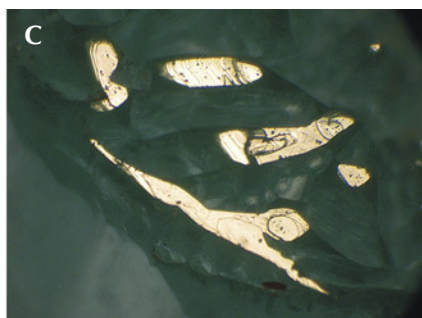
Figure 15. A: Sample 15 (37.4 mm in length), an emerald crystal with color zoning; at one end, the sample reveals a continuous rim surrounding growth areas ending in small basal faces. B: Growth and color zoning (arrows) of the crystal along the c -axis. C: Areas of the rim and small columns inside the rim with planes parallel to the basal pinacoid appear bright in reflected light, viewed parallel to the c -axis. Photos by K. Schmetzer; field of view 3.6 mm (C).
