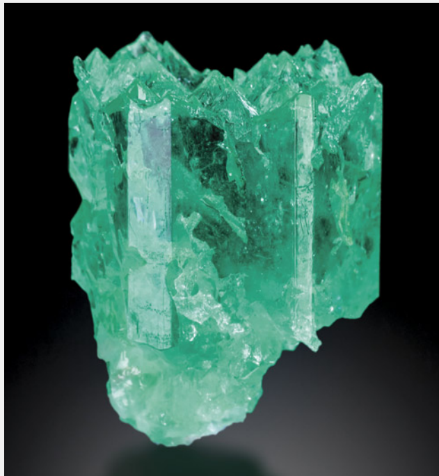
Figure A-3. Left: A heavily etched Colombian emerald crystal from Muzo measuring 27 mm in length. The basal pinacoid is completely dissolved, leading to numerous pointed hillocks; the growth sectors related to the prism faces are optically reflective. Photo by Jeff Scovil. Right: Etched beryl crystal from Pont de Barost, Haute-Vienne, France, showing a completely dissolved basal face with numerous pointed hillocks. From Lacroix (1896).
