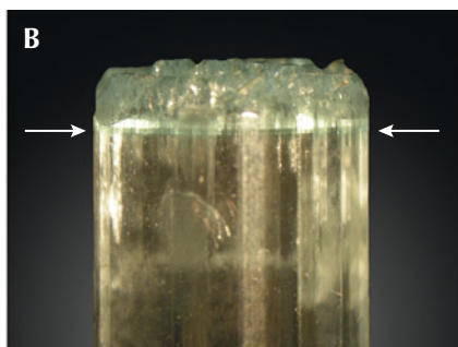
Figure 15. A: Sample 15 (37.4 mm in length), an emerald crystal with color zoning; at one end, the sample reveals a continuous rim surrounding growth areas ending in small basal faces. B: Growth and color zoning (arrows) of the crystal along the c -axis. C: Areas of the rim and small columns inside the rim with planes parallel to the basal pinacoid appear bright in reflected light, viewed parallel to the c -axis. Photos by K. Schmetzer; field of view 3.6 mm (C).
