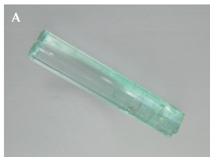
Figure 15. A: Sample 15 (37.4 mm in length), an emerald crystal with color zoning; at one end, the sample reveals a continuous rim surrounding growth areas ending in small basal faces. B: Growth and color zoning (arrows) of the crystal along the c -axis. C: Areas of the rim and small columns inside the rim with planes parallel to the basal pinacoid appear bright in reflected light, viewed parallel to the c -axis. Photos by K. Schmetzer; field of view 3.6 mm (C).
