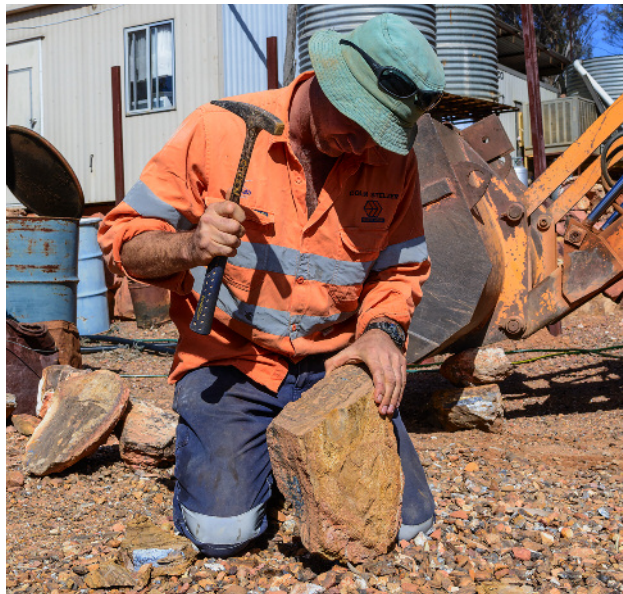
Figure 17. Boulder opal miners must split every ironstone concretion they find to reveal its contents. Photo by Andrew Lucas/GIA.
