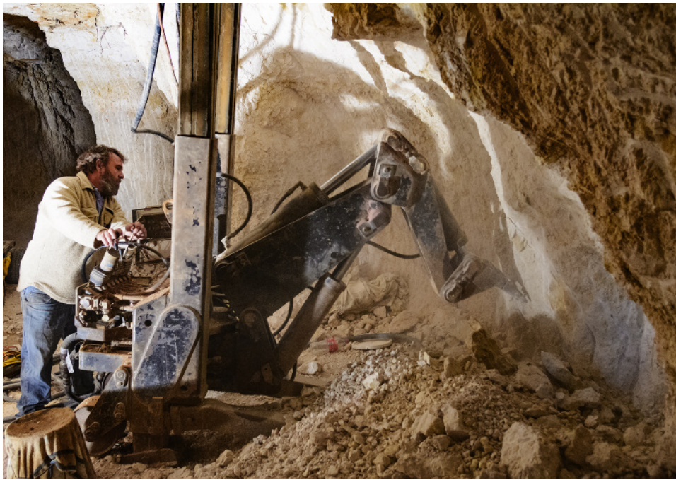
Figure 6. This customized digger is specifically designed to extract opal-bearing clay. Joints on the machine allow for greater flexibility. Photo by Andrew Lucas/GIA.
