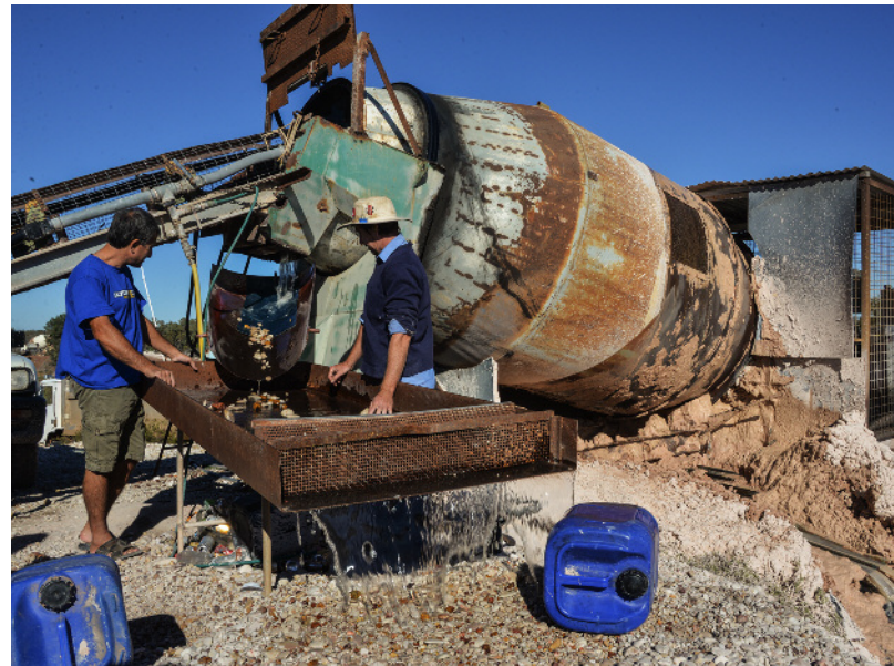
Figure 8. The agitator, a converted concrete mixer, is the core facility in the washing plant. When it rotates, the opal nodules and other materials within it circulate, removing much of the clay from the opal. Photo by Vincent Pardieu/GIA.
