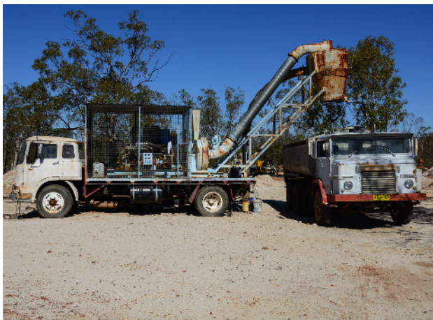
Figure 7. The “blower” is in fact a giant vacuum sucking everything mined to the surface. It is powered by a generator mounted on a truck above ground. The mined materials are loaded onto dump trucks and carried to the washing plant. Photo by Vincent Pardieu/GIA.
