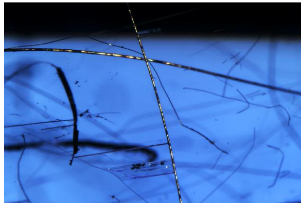
Figure 7. Merelaniite whisker inclusions in the tanzanite cabochon. Photomicrograph by Augusto Castillo; field of view 3.57 mm.
