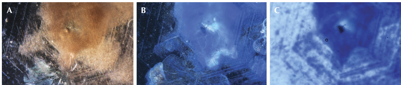
Figure 45. Example 2 before heat treatment with fiber-optic illumination (A), after heat treatment with fiber-optic illumination (B), and after heat treatment with diffuse transmitted illumination (C). Photomicrographs by Aaron Palke; field of view 4.79 mm.
