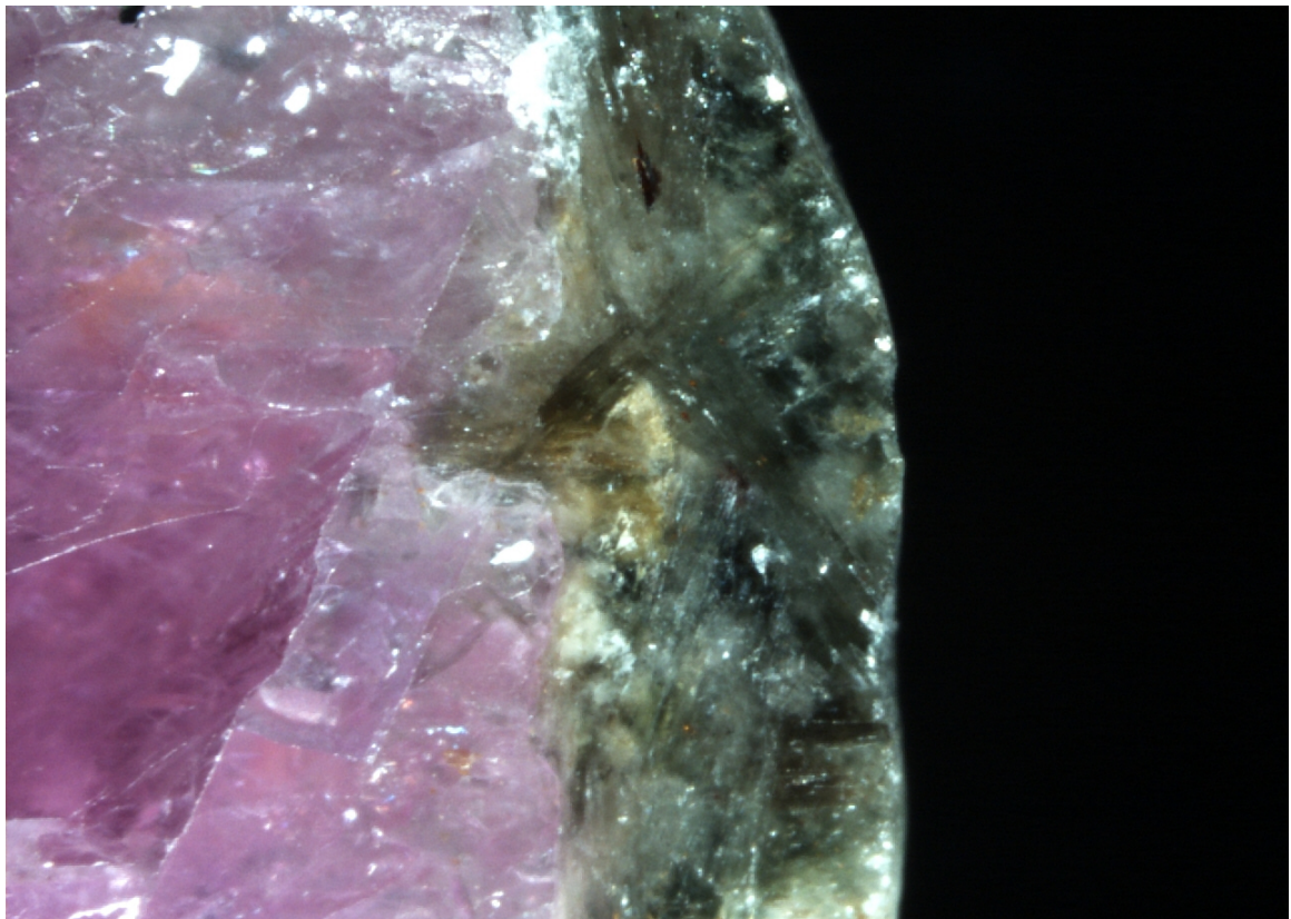
Figure 13: Green chlorite crystals on one of the ruby samples identified by Raman spectrometry.
