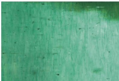
Figure 2. Thin, evenly distributed concentrations of green dye in the beryl, as seen through the table. Field of view 1.76 mm.
