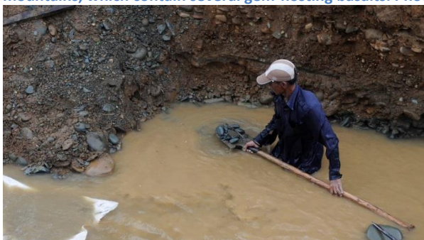
Figure 7: A miner using a long shovel to get gravel from the river bottom. Photo by Wim Vertriest-GIA.
