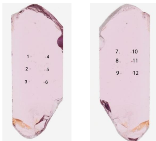
Figure 43: GIA reference sample #5902 showing the location of the 12 spots where LA-ICP-MS analysis was conducted on each side of the wafer. Photo: S. Engniwat © GIA.
