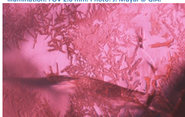
Figure 31: Epigenetic materials (boehmite and kaolinite identified by FTIR spectroscopy) in GIA reference sample 100305163680. Brightfield illumination. FOV 1.1 mm. Photo: J. Muyal © GIA.
