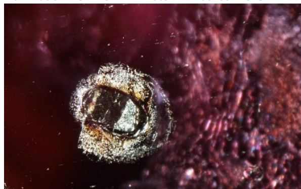
Figure 21: Using darkfield and fiber optic illumination, diopside with decrepitation halo in GIA reference sample 668835502. FOV 1.5 mm. Photo: J. Moyal © GIA.
