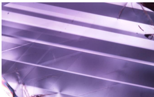
Figure 35: Polysynthetic twinning parallel to the rhombohedron in plane-polarized light in GIA reference sample 668837202. Fiber-optic light illumination. FOV 3.1 mm. Photo: J. Muyal © GIA.
