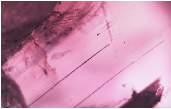
Figure 38: Growth tubules in GIA reference sample 100310677106. Brightfield illumination. FOV 1.2 mm. Photo: V. Raynaud © GIA.
