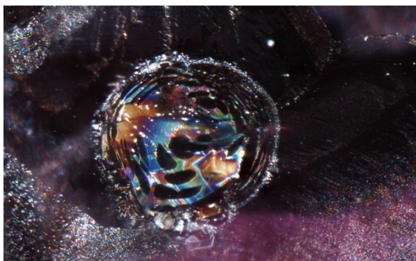
Figure 14: Fluid fingerprint in GIA reference sample 100305163702. Fiber-optic light illumination. FOV 1.1 mm. Photo: J. Muyal © GIA.
