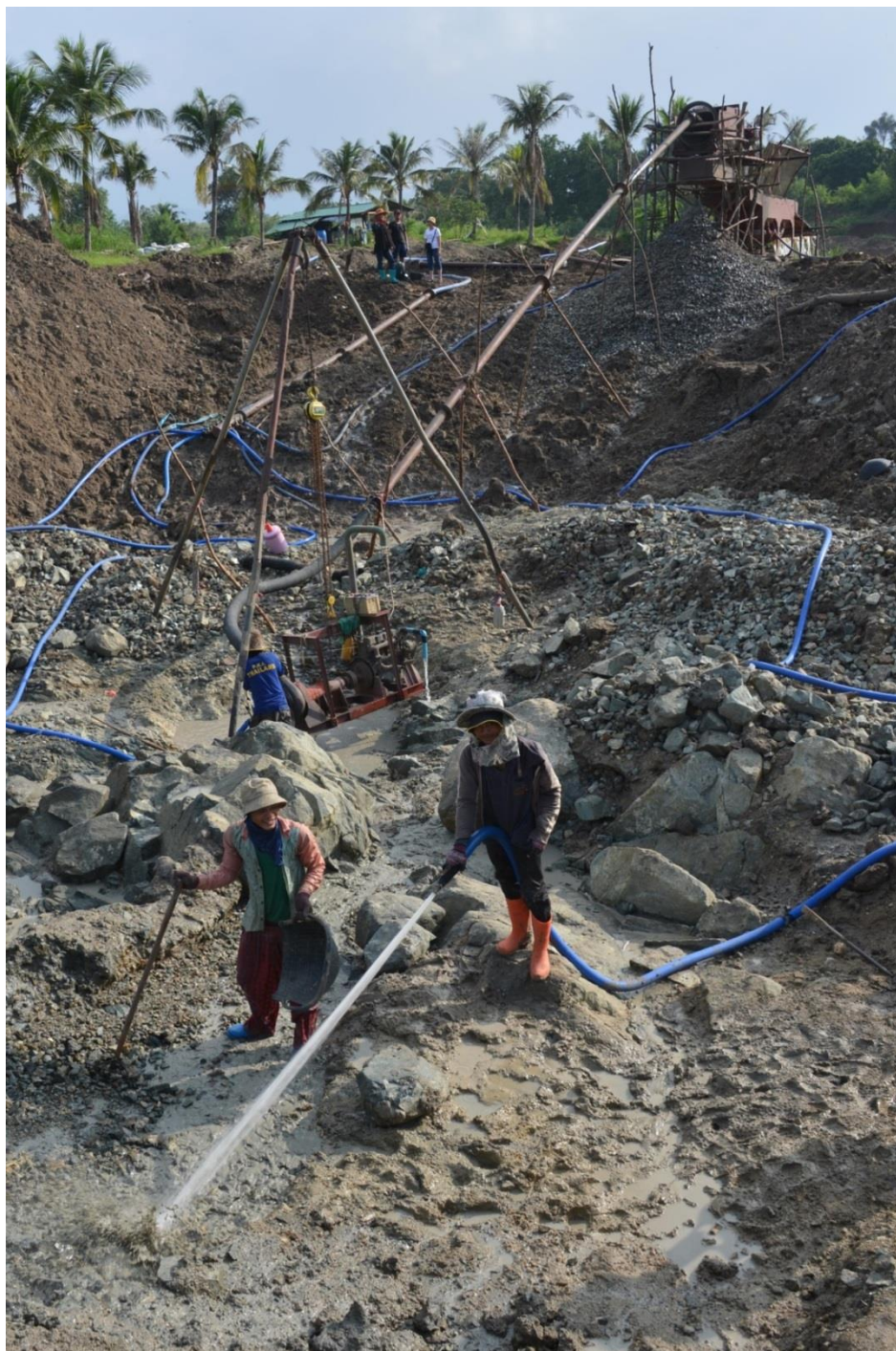
Figure 5: Mining old river deposits near the Pailin river. From bottom to top, we can see: Miner working high pressure waterjet to loosen the gravels; gravel pump to move the slurry; jig to concentrate the minerals. Photo by Vincent Pardieu-GIA.
