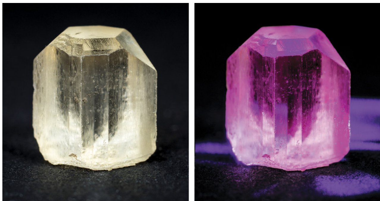
Figure 9. Two photos of the second crystal from the left in figure 3 (1.6 g, 9.5 mm tall). Left: White-light photo showing the common pale yellow bodycolor. Right: The crystal emits pink to red luminescence under 407 nm illumination. Photos by Manfred Wildner.
