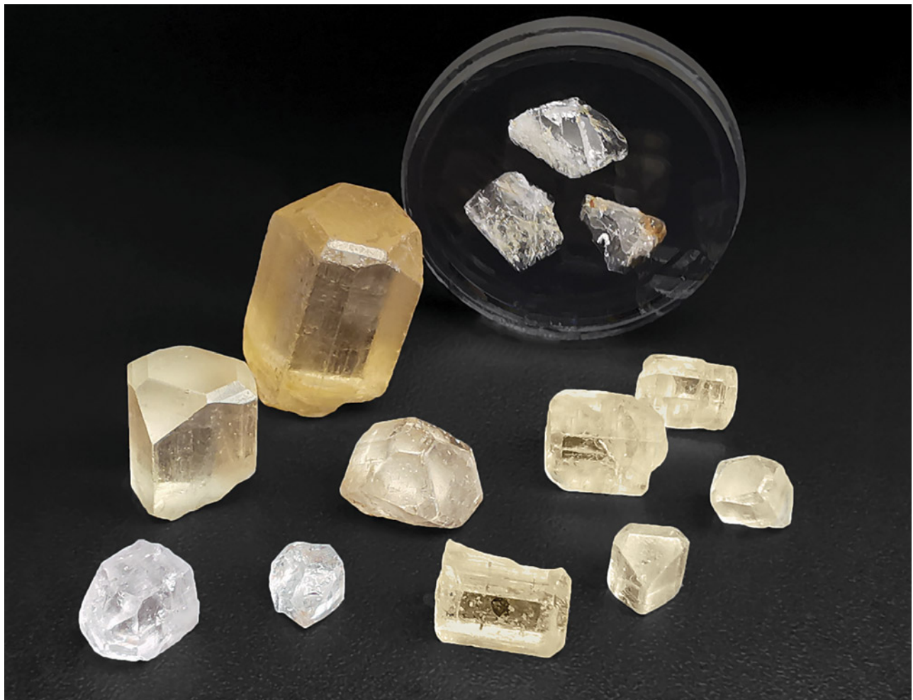
Figure 3. Topaz sample material investigated in the present study (height of the tallest crystal is 18 mm). The two colorless samples (lower left) were initially yellow and became bleached upon heat treatment at 550°C for 48 h. The one-inch sample mount in the background contains three doubly polished crystals embedded in epoxy; it was subjected to spectroscopy, EPMA, and LA-ICP-MS analysis. Photo by Manuela Zeug.
