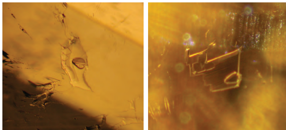
Figure 4. Multiphase inclusions, consisting of a single bubble and three crystals in a watery solution, were observed in grossular from Itrafo. Photomicrographs by I. Adamo; magnified 60 \times (left) and 65 \times (right).
