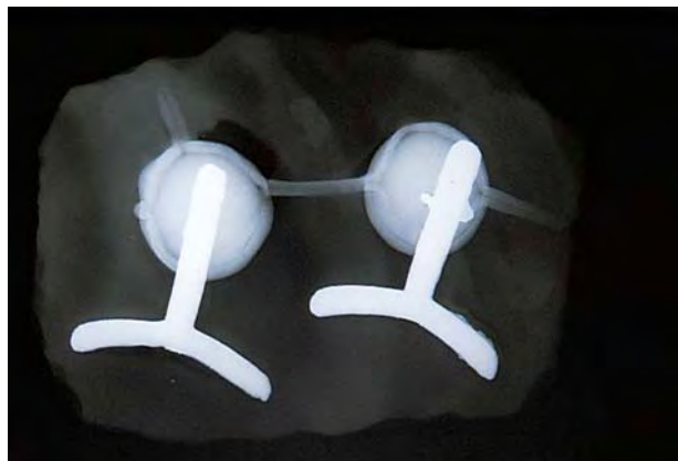
Figure 3. This X-radiograph of pearls cultured by Carl V. Linne in 1761 reveals two shell beads that are strung together with thread (as in the Chinese example in figure 2). The cultured pearls are separated from the shell surface by two T-shaped metal posts. In this manner, Linne produced cultured pearls that were almost entirely coated with nacre. Specimen loaned to Fred Woodward by the Linnaeus Society, London.
