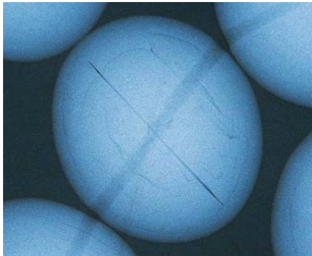
Figure 11. Concentric rings, related to the growth of this 10–11 mm Chinese FWCP, can be seen circling the elongate implant line in the center and a smaller implant “core” to the right. Note, however, that the central implant line takes up approximately 80% of the diameter of this FWCP, crossing some of the concentric lines, so the presence of a bead or cultured pearl nucleus would be impossible.
