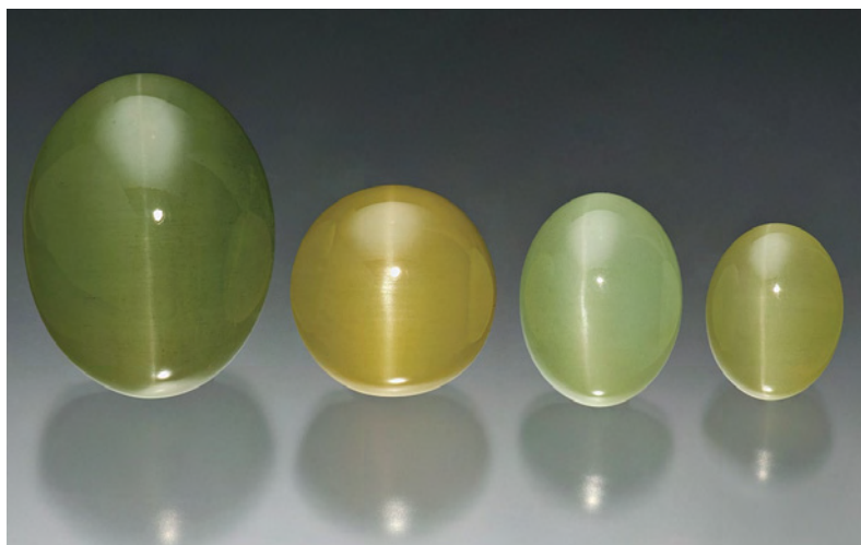
Figure 3. These cat's-eye beryl cabochons (46.76–282.63 ct), reportedly from Shahpura in India's Rajasthan State, show a sharp chatoyant band oriented perpendicular to the c-axis. Photo by Robert Weldon; the 46.76 ct stone (far right) is GIA Collection no. 37971.
