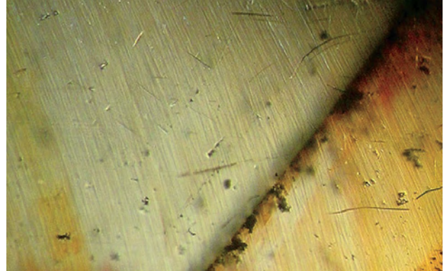
Figure 17. Polish lines on the bases of the sphaerulite cabochons were responsible for the phenomena. Photomicrograph by J. Hyršl; field of view 2 mm.
