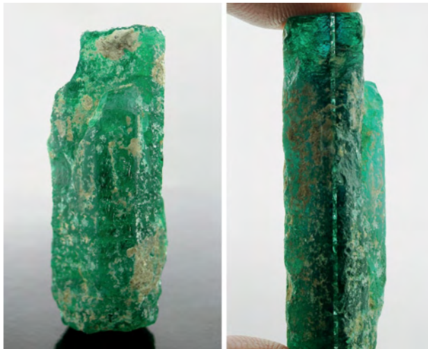
Figure 22. This ~21.8 g sample, represented as natural emerald from Russia, proved to be a cleverly fashioned hydrothermally synthetic. The view on the right reveals the presence of a colorless seed plate. Photos by S. Singbamroong, © Dubai Gemstone Laboratory.
