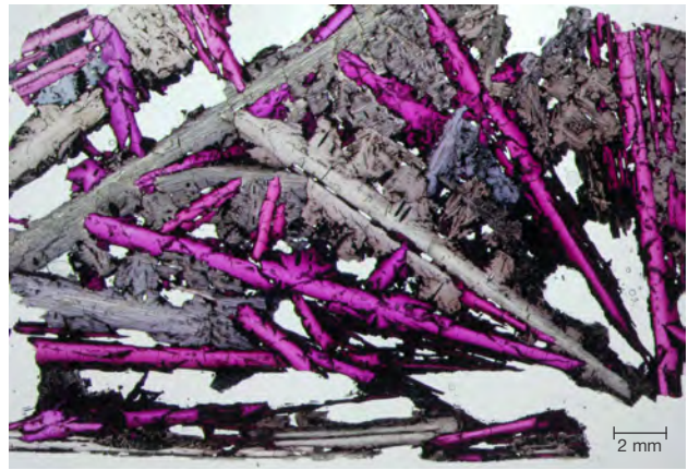
Figure 15. Photomicrograph of a petrographic thin section of ruby (purplish red)-diaoyudaoite (grayish green) slag, shown in transmitted light. From Sorokina et al. (2010).
