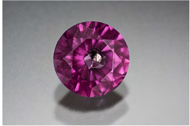
Figure 13. The prominent sulfide inclusion in this 2.02 ct pyrope is clearly visible under the table facet. Photo by Kevin Schumacher.
