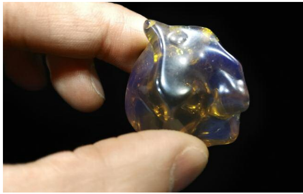
Figure 23. This 139.34 ct piece of artificial glass bore a striking similarity to blue amber. Photo by Lai Tai-An Gem Lab.
