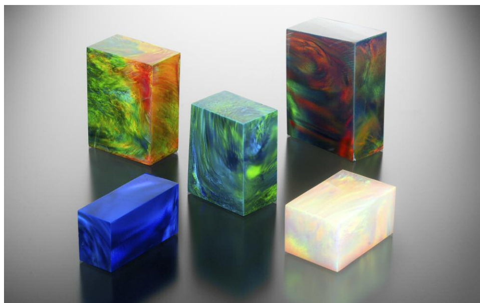
Figure 30. This opal imitation shows a bilowy play-of-color phenomenon. The largest block measures approximately 61.79 mm in length. Photo by Robison McMurtry and Diego Sanchez. Courtesy of Sanwa Pearl & Gems Ltd.
