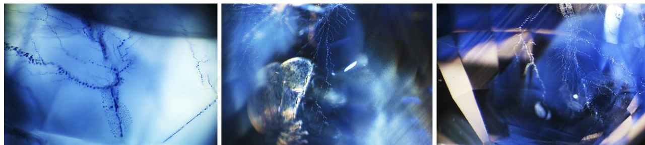
Figure 33. Left: Dendritic inclusions consisted of dot-like minerals showing a “melted and diffused” appearance. Photo by Yujie Gao; field of view 2.68 mm. Center: Resembling a tree root, these dendritic inclusions showed relatively strong metallic luster under reflected light. Photo by Yizhi Zhao; field of view 2.52 mm. Right: Dendritic inclusions coupled with blurred blue color zoning. Photo by Yujie Gao; field of view 9.73 mm.
