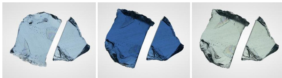
Figure 10. Two wafers of the new Nigerian aquamarine in unpolarized light (left), and with light polarized along the extraordinary ray (center) and along the ordinary ray (right). Photos by Aaron Palke.
