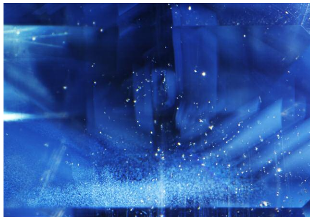
Figure 62. Zircon crystals scattered throughout angular milky clouds were more prominent in these sapphires compared to other high-Fe sapphires. Photomicrograph by Jessa Rizzo; field of view 4.7 mm.
