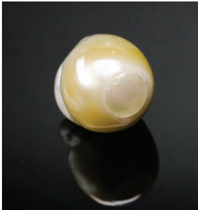
Figure 8. The 10.27 ct baroque cultured pearl exhibited a suspicious translucent ring at one end.
