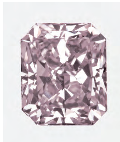
Figure 4. This 1.42 ct type IIb natural diamond was significant for its unusual Fancy gray-purple color and its strong emission at 776.4 nm under PL spectroscopy.
