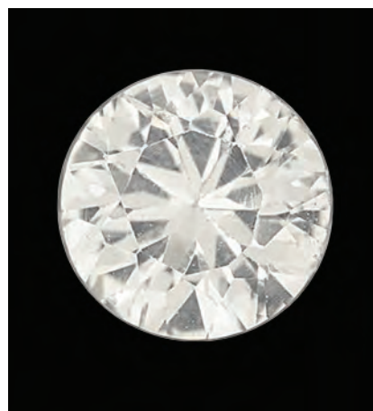
Figure 22. Left: The 1.14 ct synthetic sapphire under daylight-equivalent lighting. Right: The sample exhibited phosphorescence in this DiamondView image.
