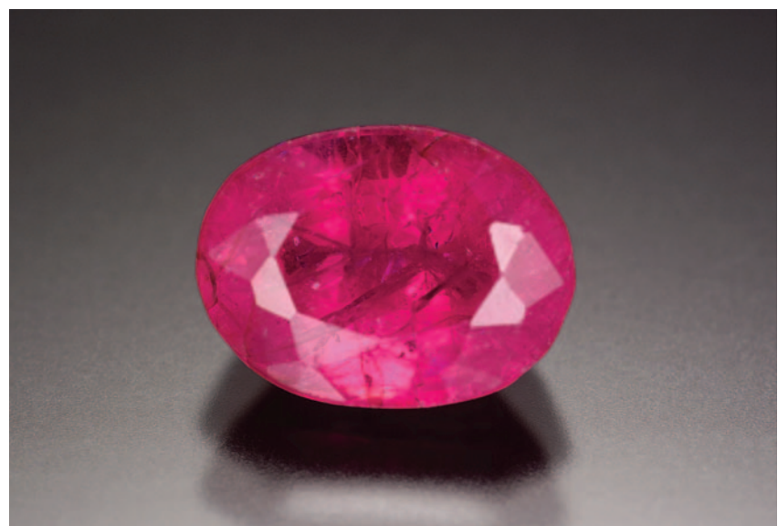
Figure 23. This 3.53 ct laboratory-grown ruby was treated with lead-glass filling.
