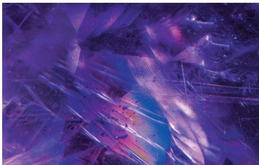
Figure 10. Iridescent cleavage cracks and needle-like structures were present in the faceted hexagonite. Field of view 3.50 mm.
