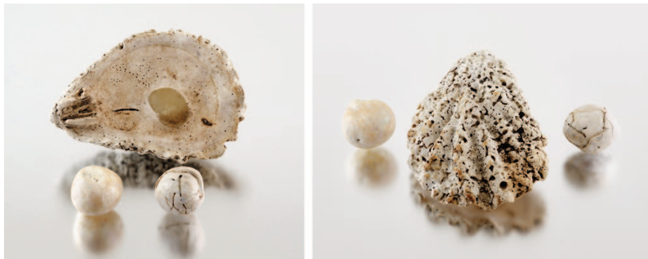
Figure 21. Three fossilized specimens recently submitted to GIA's New York laboratory: two fossil pearls (12.64 × 11.50 × 10.00 mm and 13.08 × 11.45 × 10.18 mm, left and right, respectively) and a fossil shell (45.97 × 32.03 × 10.90 mm) containing a shell blister. Courtesy of Kathryn Malatino and Aaron Brown.
