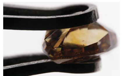
Figure 6. Fancy Vivid orange color distribution with strong zoning related to crystal growth.
