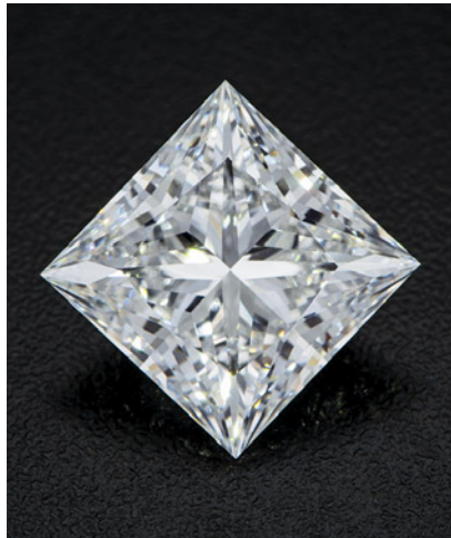
Figure 15. This 15.73 ct G-color CVD-grown diamond showed indications of HPHT treatment.
