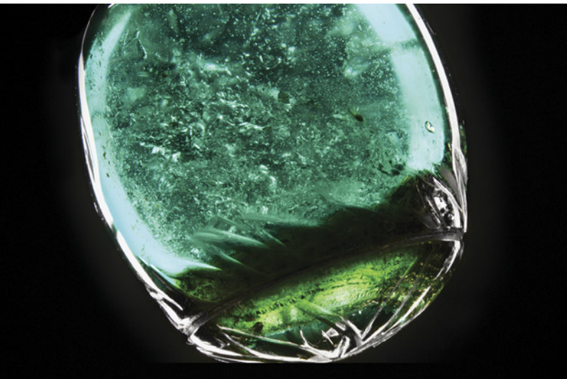
Figure 17. The assemblage appears as two carved pieces attached to the setting with a green cement. Colorless gas bubbles can be observed, an indication that this piece is not what it seems. Photomicrograph by Ezgi Kiyak; field of view 21.2 mm.
