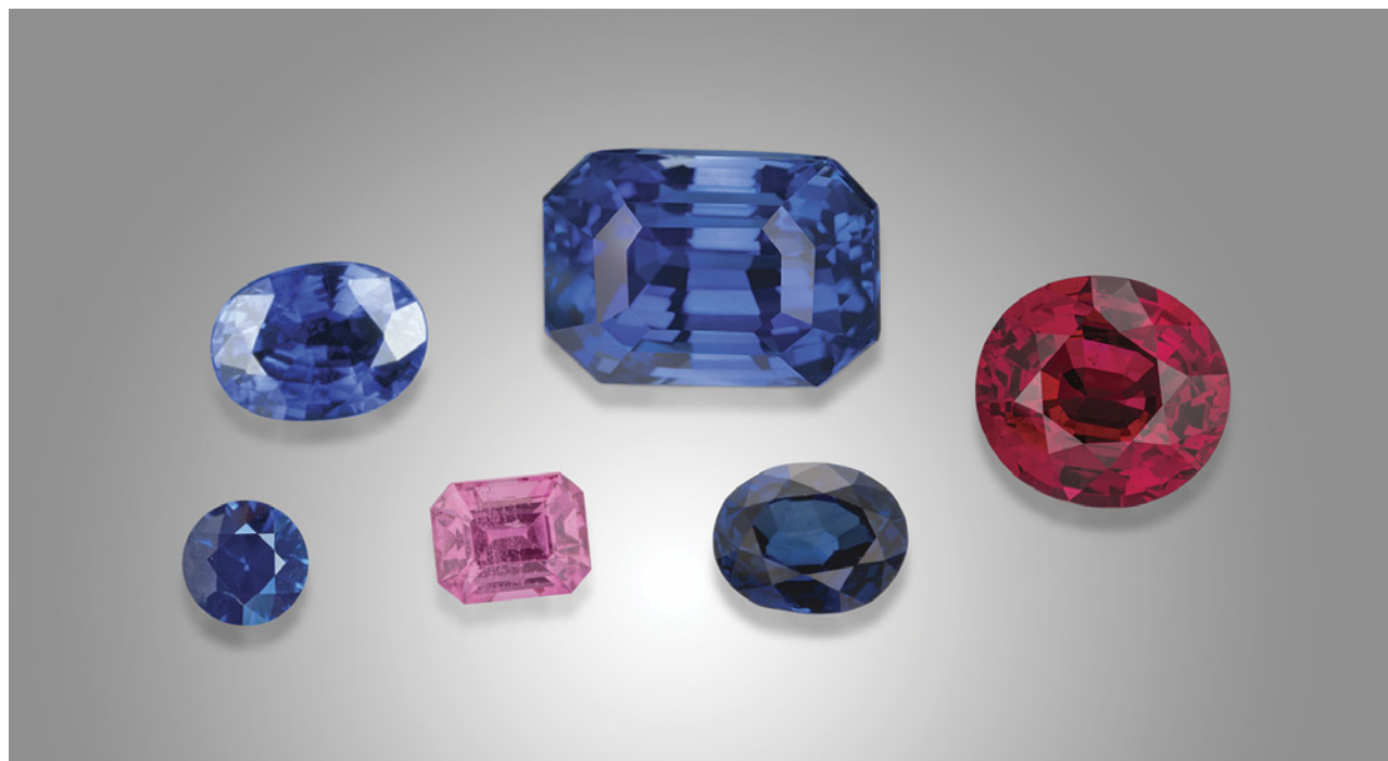
Figure 11. Various types of corundum (ranging from 1.16 to 33.16 ct) that can present the 3309 \text{cm}^{-1} series in FTIR spectra: unheated basalt-related blue sapphire (two stones in the bottom row), heated metamorphic blue sapphire (two stones in the top row), and pink sapphire and ruby. Photos by Robert Weldon, Orasa Weldon, Vincent Pardieu, Emily Lane, and Tino Hammid; stones courtesy of B&B Fine Gems, Kenneth Kin Ming Siu, and Joao Jose Ip Lau Tchun.
