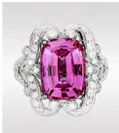
Figure 21. This pink stone proved to be a flux-grown synthetic sapphire with unusual crystal inclusions.
