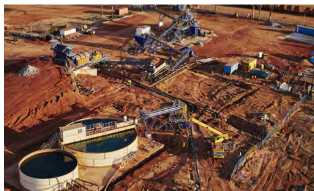
Figure 11. An aerial view of MRM's new ruby washing plant, which uses dense media separation. Photo courtesy of Gemfields.
