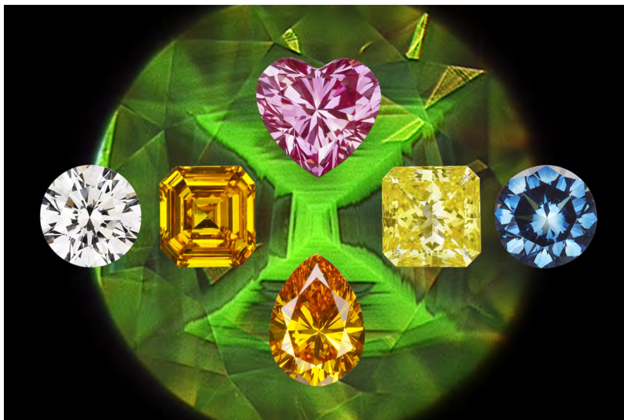
Figure 1. This collection of HPHT synthetics shows the major color products. The background is a DiamondView image with a cross-shaped fluorescence pattern, a well-known diagnostic feature of HPHT synthetics.
