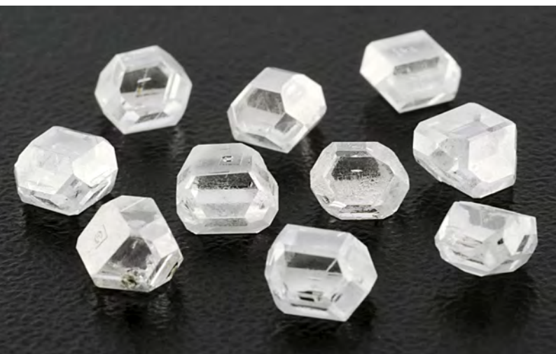
Figure 2. This selection of colorless HPHT synthetic crystals (0.50–0.69 ct) was grown by Jinan Zhongwu New Materials Company Ltd. of Shandong, China.
