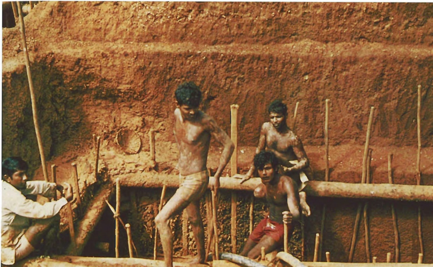
Figure 5. Two to three meters below ground level, the gem-bearing gravel is extracted by workers. Natives use picks and shovels to excavate the gem gravel, a common practice in pit mines in the Elahera field.
