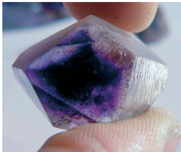
Figure 7. This crystal from Boudi displays the classic morphology of amethyst. Clearly visible is the habit of the hexagonal prism and the two different rhombohedra (positive and negative). The hematite inclusions, mainly oriented perpendicular to the surface of the prism, are clearly visible in the outer colorless portion. Photo by Abdelghani El Harfi and Salahaddine Mouaddib.
