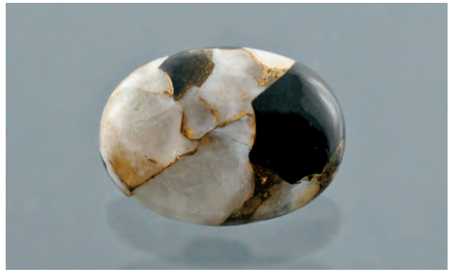
Figure 9. This 8.54 ct cabochon was a composite of brown opal and white calcite. Photo by G. Choudhary.
