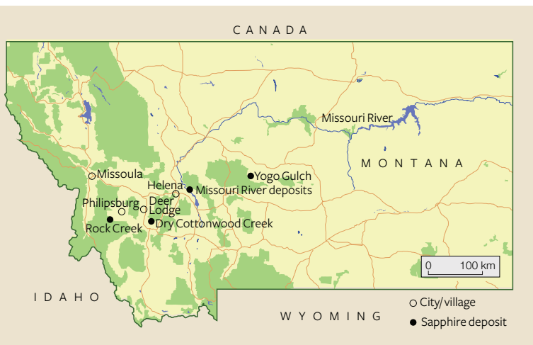
Figure 1. Locations of sapphire deposits in the U.S. state of Montana. Yogo Gulch is the only primary deposit, while Rock Creek is the most important alluvial deposit.
