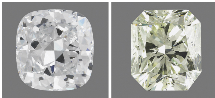
Figure 18. These two large synthetic diamonds were produced using HPHT growth methods by the Russian firm New Diamond Technology. The 4.30 ct specimen on the left has D color and SI 1 clarity. On the right is a 5.11 ct sample with K color and I 1 clarity.
