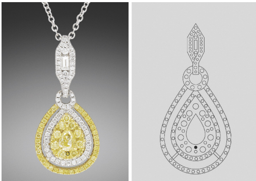
Figure 16. A photo and a detailed illustration of the melee-set pendant show the location of all 118 samples. The single HPHT synthetic melee is highlighted in both images.
