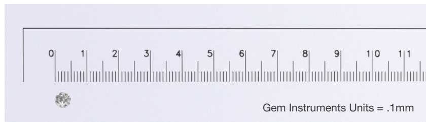
Figure 4. This 0.00054 ct colorless round brilliant was submitted for identification as a natural or synthetic diamond. Despite the specimen's small size, an FTIR microscope can focus a beam through the facets to capture a high-quality infrared spectrum.
