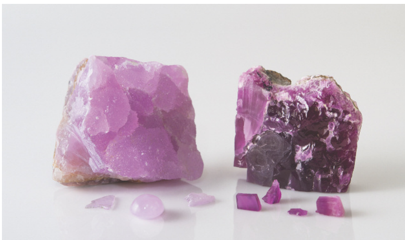
Figure 1. The pink and reddish purple cobaltocalcite specimens (246.3 and 361.0 g, respectively) are shown with some of the wafers cut from them.
