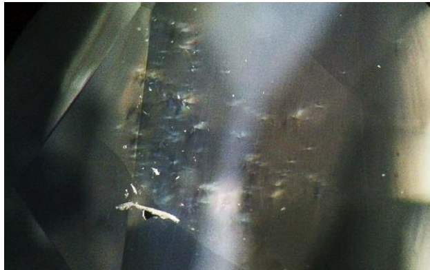
Figure 16. These small stress points, visible on the table between crossed polarizers, were confined to a small space. Photomicrograph by Meenakshi Chauhan; magnified 30x.
