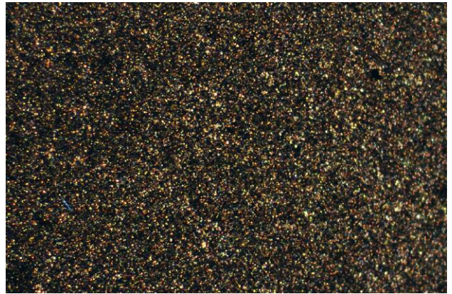
Figure 8. Under reflected light, the boron carbide specimen displayed a dense, fine granular structure typically associated with aggregates such as ceramics. Photomicrograph by Gagan Choudhary; magnified 48x.
