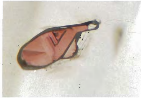
Figure 3. Trigons, which are typical of a diamond octahedron, can be seen on the face of this flattened inclusion of pyrope garnet, with a colorless enstatite (orthopyroxene) or olivine crystal at the end. These features are taken as evidence that the diamond has forced its crystal habit on the guest mineral during the simultaneous crystallization of inclusion and host. Photomicrograph by Eduard J. Gübelin; transmitted illumination, magnified 50 \times . From Gübelin and Koivula (1986, p. 95).
