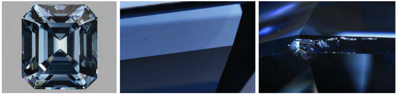
Figure 13. A 5.03 ct Fancy Deep blue HPHT synthetic diamond was examined by GIA (left). Faint but sharp color zoning was observed (middle, field of view 4.77 mm), along with small metallic inclusions and a cavity at the girdle (right, field of view 2.19 mm).
