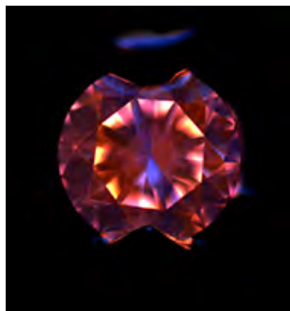
Figure 17. DiamondView imaging showed strong orange fluorescence with small irregular areas of blue fluorescence, a typical feature of as-grown CVD synthetic diamond.
