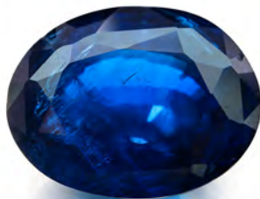
Figure 18. A 9.75 ct synthetic spinel, seen in GIA's Bangkok lab, was proven to be treated by the quench-crackling method.
