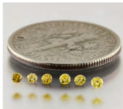
Figure 4. These six melee were revealed to be HPHT-treated natural diamonds.
