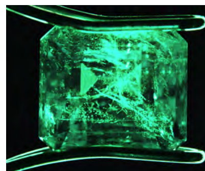
Figure 7. This 1.81 ct specimen was a natural emerald/emerald doublet. Field of view 10.5 mm.
