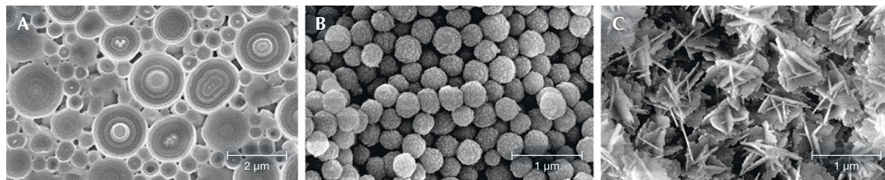
Figure 3. SEM images showing the silica spheres in common opal. Instead of solid concentric spheres (A and B), opal-CT and opal-C may contain lepispheres (spherical aggregates of blades, C). The spheres in common opal scatter light completely randomly due to the irregular arrangement, creating the typical milky appearance. The sizes of the silica spheres in common opal may cover a wide range (A) or be very similar to each other (B and C). Image A from Gaillou (2015) and B and C from Gaillou et al. (2008).
