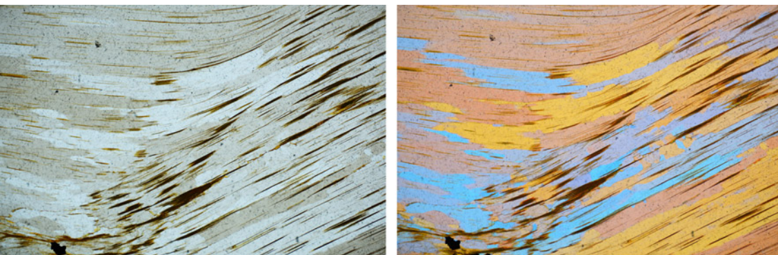
Figure 18. Thin section of tiger's-eye under cross-polarized light (left) and with a lambda plate inserted to enhance the contrast across grain boundaries (right). The dark brown needles are the iron oxide/hydroxide from weathered amphibole. Photomicrographs by Amir C. Akhavan; field of view 1.5 mm.
