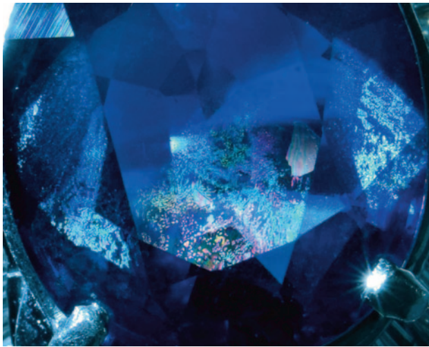
Figure 10. Large iridescent healed fissures in an oval mixed-cut sapphire. Photo by Shunsuke Nagai; field of view 12.20 mm.
