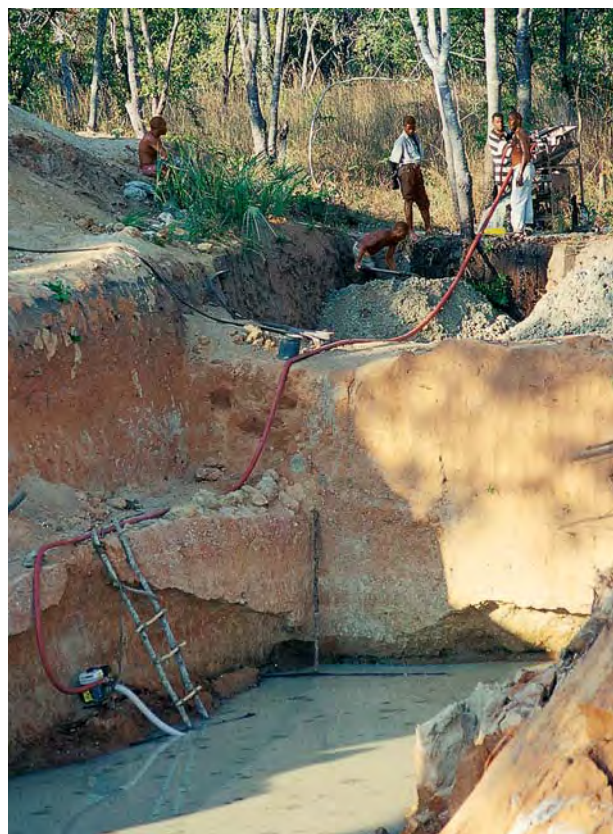
Figure 14. Large quantities of garnets—in several varieties—were recovered from the Tunduru area of Tanzania. The mines are worked by simple methods, as shown by this pit at Libafu. A portable wet-sieving machine is being used to concentrate the gem rough. Photo by Horst Krupp.
