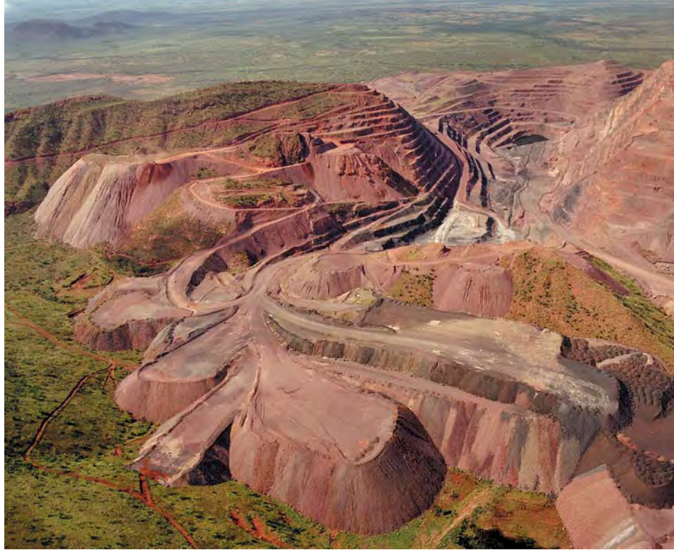
Figure 10. This aerial view of the Argyle diamond mine in northern Australia, taken in February 2000, shows the enormous open pit and tailings piles. During the past decade, this mine has been the world's largest producer of diamonds by volume. Courtesy of Argyle Diamonds.
