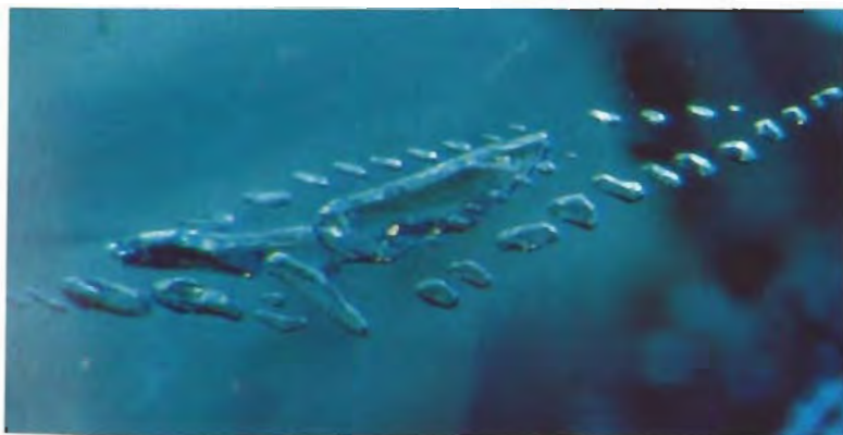
Figure 19. Negative crystals were common in the Andranondambo sapphires. Here, large, elongated negative crystals are accompanied by a "seam" of smaller ones. Magnified 80X.
