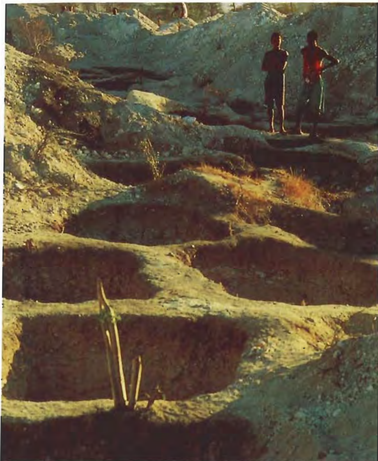
Figure 6. At the Andranondambo mining area, it is dangerous to walk between the deep shafts, which are sometimes not more than 50 cm apart. Note in the shafts the profile of the cataclastic structure of the calcareous sapphire-bearing rock. Photo by E. J. Petsch.
