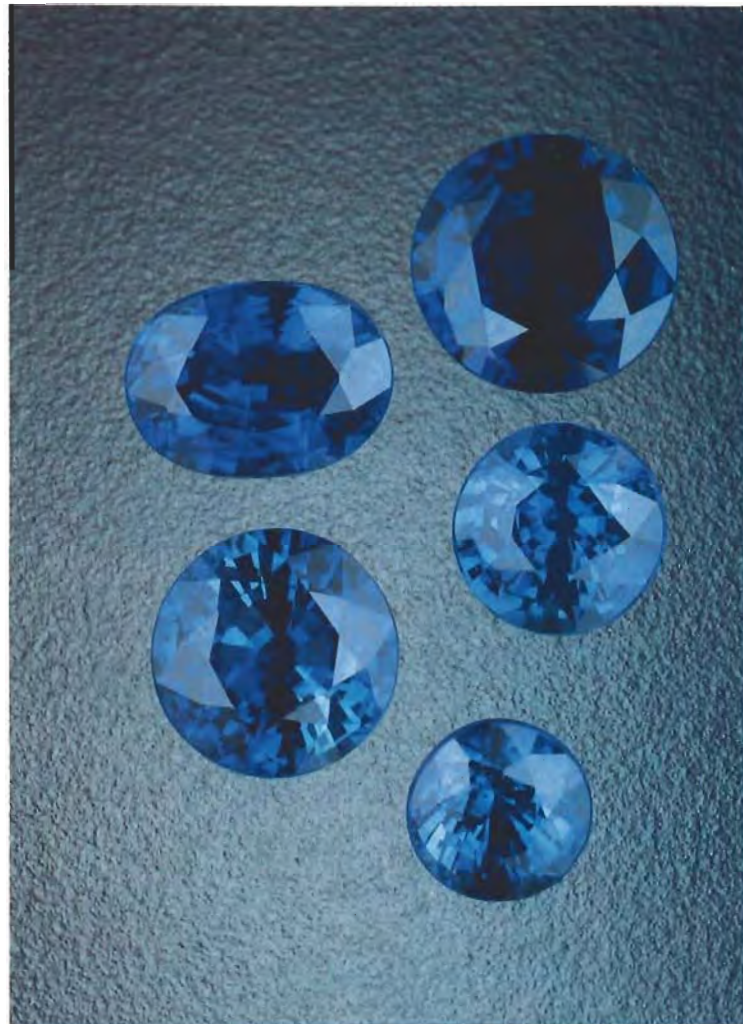
Figure 9. Heat-treated sapphires from southern Madagascar (like these 0.28–0.57 ct stones) typically range from medium dark to dark blue. Courtesy of heat treaters Kenneth Kin Ming Siu and Joao Jose Ip Iau Tchun; Photo © GIA and Tino Hammid.
