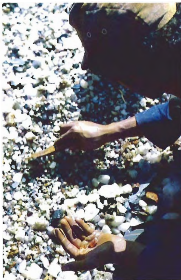
Figure 7. Hand sorting the residual "heavies" for topaz.
