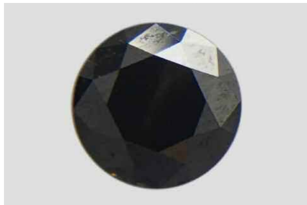
Figure 11. This 1.03 ct opaque round brilliant cut with a striking pattern of micro-inclusions was identified as a black diamond. Photo by Yujie Li.
