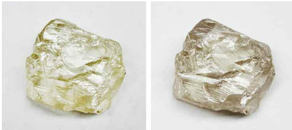
Figure 16. The Foxfire under ambient room lighting, before (left) and just after exposure to long-wave UV light (right). Photos by Jeffrey Post.
