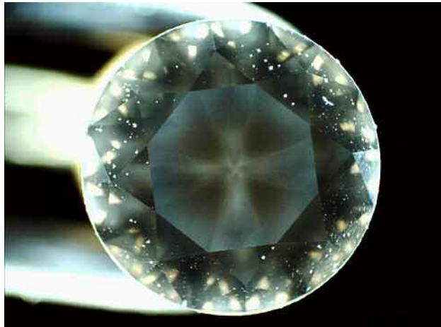
Figure 12. The “double cross” pattern seen in the black diamond. This pattern showed that the small inclusions were restricted to certain sectors, indicating that the diamond crystallized through two separate processes. Photo by Yujie Li; field of view approximately 4 mm.
