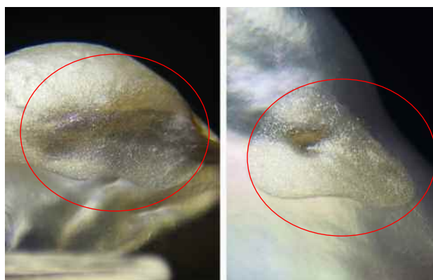
Figure 24. Two fillings displayed a coarse appearance and lower luster that differed from the rest of the pearl. Photomicrographs by Lai Tai-An Gem Lab; fields of view 11.5 mm (left) and 8.6 mm (right).
