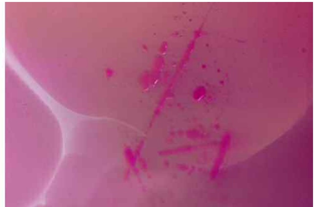
Figure 29. Both the blue and pink opal showed dye color concentrations around pits and scratches on the surface, consistent with hydrophane opal that has been artificially dyed. Photomicrographs by Nathan Renfro; fields of view 2.34 mm (left) and 1.99 mm (right).
