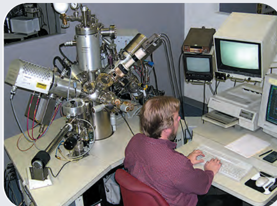
Figure A-1. Shown here is a SIMS instrument in use at Evans East. This PHI 6600, manufactured by Physical Electronics, employs a quadrupole mass spectrometer to detect and sort ions from the corundum sample.
