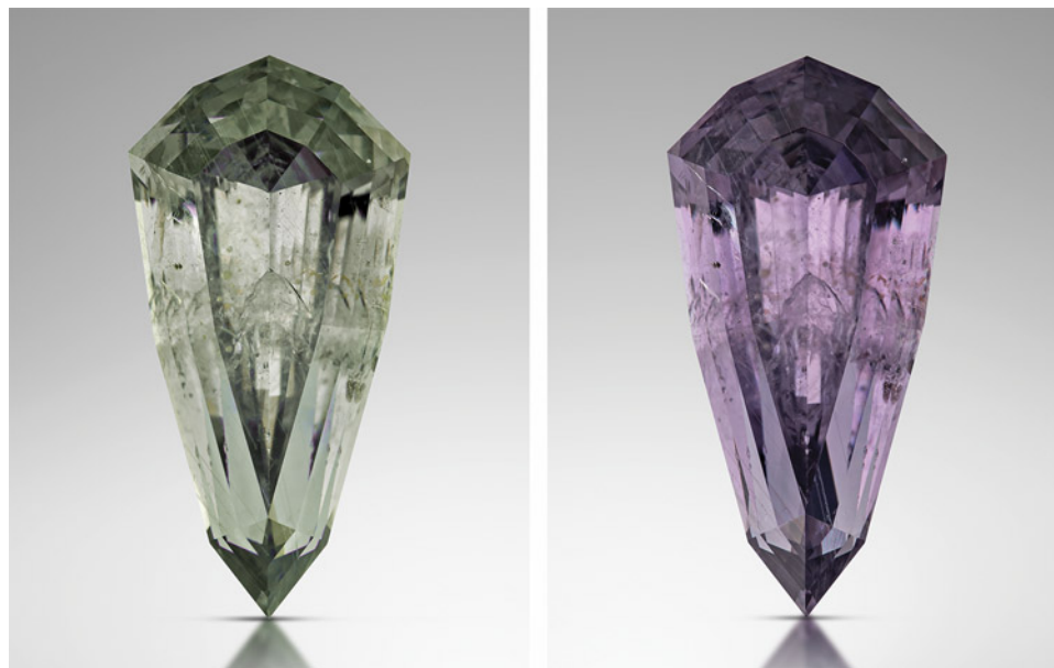
Figure 17. A strong color change—going from bluish green to pinkish purple—is observed in this 3.49 ct French Bar sill sapphire (RK-FBS 030; also shown in figure 2) with a change from fluorescent (5500 K, left) to incandescent light (2800 K, right). Photos by Jeff Mason.
