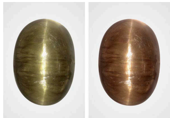
Figure 9. The 60.71 ct diaspore displaying color change and chatoyancy under fluorescent light (left) and incandescent light (right).
