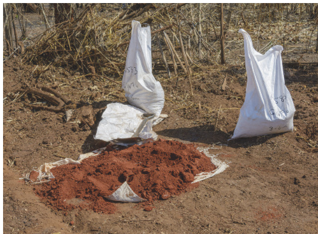
Figure 12. These bags of gravel layers will be transported to the washing plant and then to the sorting house. This will give a reasonable estimation of ruby concentration. Photo by Andrew Lucas/GIA.
