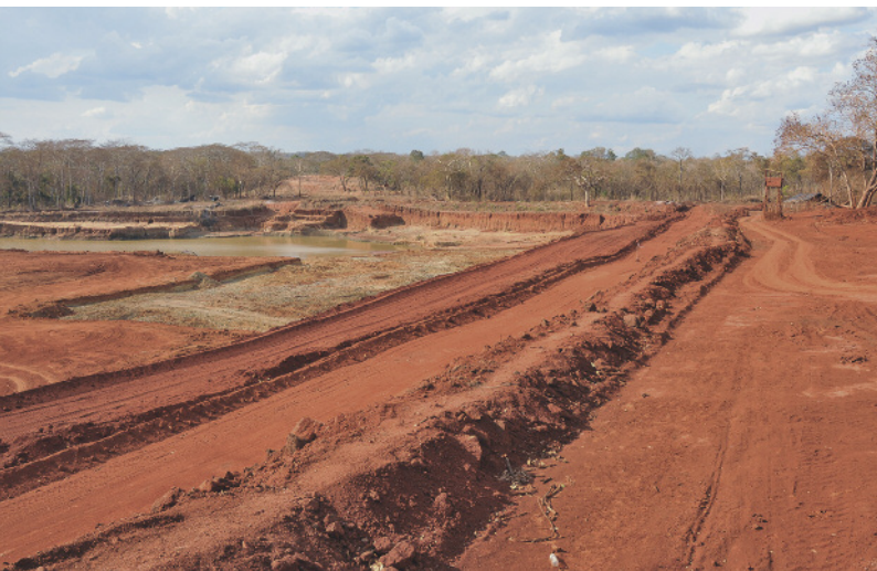
Figure 7. This photo shows the bulk sampling pit in Maninge Nice. The greenish layer is the weathered ruby-bearing amphibolite, and the contact between the topsoil and the amphibolite is visible. Photo by Vincent Pardieu/GIA.
