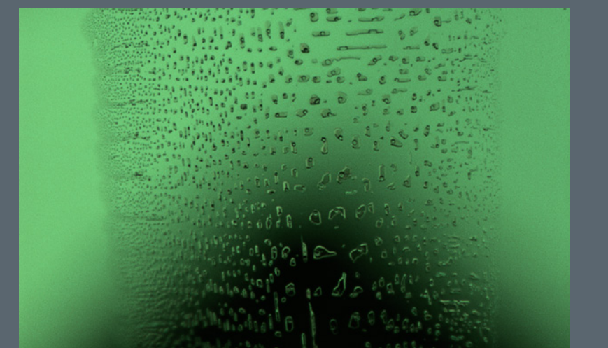
Flux residue often contains a contraction bubble, as seen in each of these trapped flux droplets. Field of view 1.08 mm.
