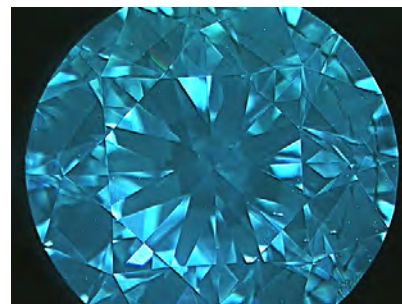
Figure 18. This DiamondView image of the 1.60 ct HPHT synthetic shows the diagnostic square pattern seen in the crown facets.
