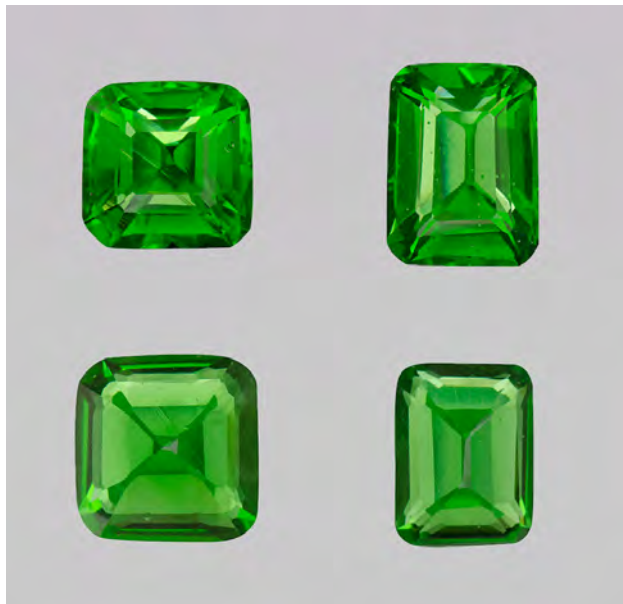
Figure 8. Face-up (top) and face-down (bottom) views of the imitation moldavite examined in this study. The sample on the left weighs 3.80 ct (9.48 × 9.30 × 6.93 mm); the specimen on the right is 3.76 ct (10.76 × 8.11 × 6.02 mm). Testing identified them as “soda-lime” glass. Photos by Nuttapol Kitdee.
