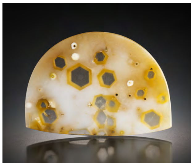
Figure 1. Measuring 52.56 \times 36.71 \times 2.88 mm, this half-moon-shaped chalcedony plate contains more than a dozen hexagonal quartz windows. Photo by Kevin Schumacher.
