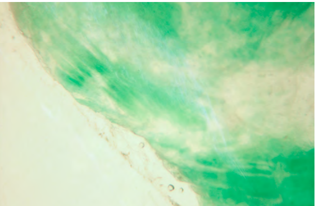
Figure 18. Left: The green color on this jadeite appears to float on the surface and has a clear boundary. Field of view 5.50 mm. Right: Resin with bubbles fills the space in the contact area. Field of view 16.8 mm. Photomicrographs by Shufang Nie.
