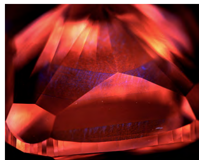
Figure 12. Fluorescence imaging from the DiamondView showed strong red fluorescence with bundles of violet-blue. Up to six growth layers basically parallel to the table were revealed.
