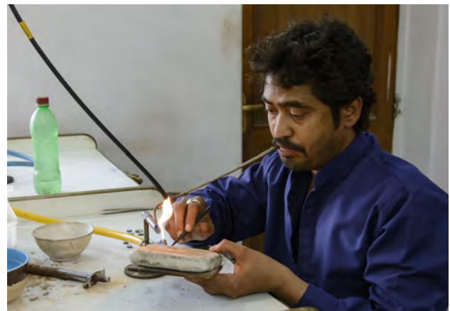
Figure 30. Even today, many of Gem Palace's master goldsmiths prefer soldering with a blowpipe, which they feel controls the flame and heat more precisely than a modern torch. Photo by Andrew Lucas, courtesy of Gem Palace.
