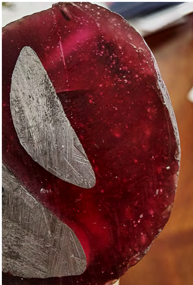
Figure 14. Air bubbles are randomly scattered in various portions of the resin matrix. Photo by Emanuele Costa.
