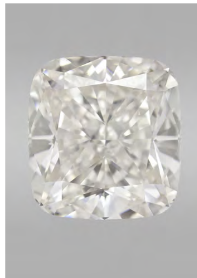
Figure 9. This 5.19 ct CVD-grown diamond ( 10.04 \times 9.44 \times 6.18 mm, with J-equivalent color and \text{VS}_2 -equivalent clarity) is the largest CVD synthetic GIA has identified to date.
