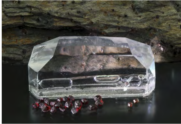
Figure 9. A 50 × 27 × 13 mm synthetic quartz crystal in which almandine and pyrope garnets introduced during the growth process created a suite of inclusions in the lower right of the specimen within the same plane as an elongated liquid and gas two-phase inclusion. The six vertical prism faces and angled rhombohedral faces help orient the crystal and mirror those of natural quartz, but their unnatural surface features immediately give away the synthetic origin. In the foreground are approximately 2.5 mm water-worn pyrope crystals (left) and 1.5–2.0 mm dodecahedral almandine crystals (right) similar to those used as inclusions; the almandines were extracted from the schist matrix specimen shown in the background. Photo by Elise A. Skalwold.
