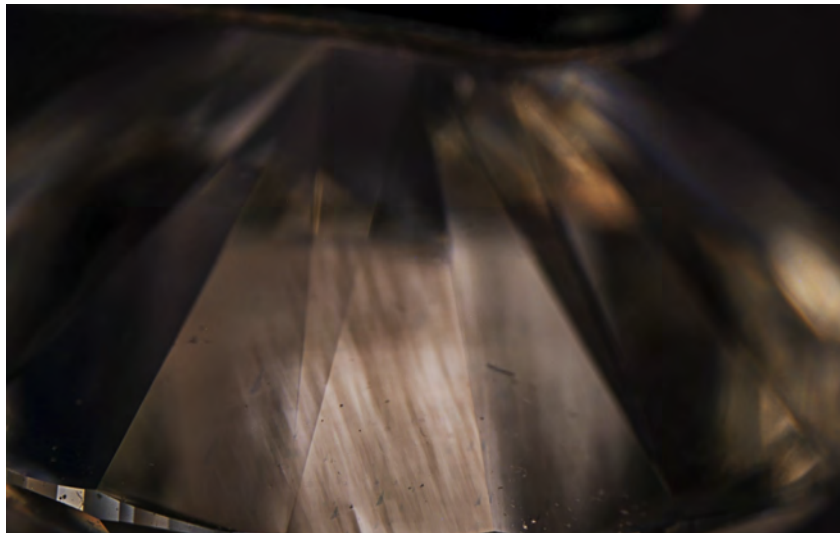
Figure 19. An image taken with polarized light showing the linear birefringence colors, indicating the presence of linear strain in the diamond lattice. Field of view 6 mm.
