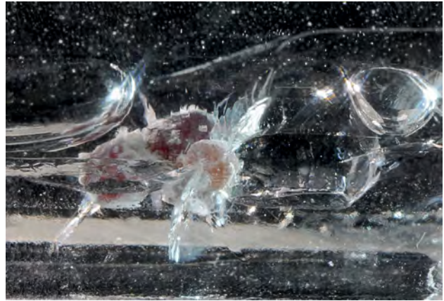
Figure 10. Amid a storm of breadcrumb inclusions, two orangy red almandines and two larger red pyropes caused tension cracks to form in the quartz upon cooling. Portions of a two-phase liquid and gas inclusion running nearly the length of the crystal are indicated by the large bubbles seen at the left and right edges of the image. The guest quartz crystal (part of a multi-phase inclusion at right), along with the white masses accompanying the garnets, are remnants from the nutrient environment in which the quartz crystal grew. Transmitted and oblique fiber-optic light. Photo by Elise A. Skalwold; field of view 13 mm.
