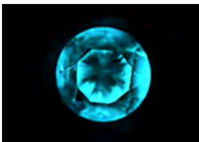
Figure 17. Phosphorescence in an HPHT-grown synthetic diamond melee.
