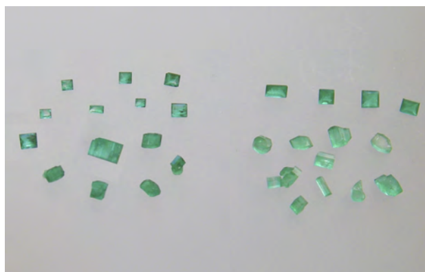
Figure 4. Rough and faceted synthetic emeralds grown by Nacken in the mid-1920s from molybdenum-bearing fluxes (type 1, left) and from molybdenum- and vanadium-bearing fluxes (type 2, right). Colorless seeds are observed with the unaided eye in many of the samples. The largest crystal, in the center left, weighs 0.51 ct and measures 5.5 × 3.5 mm. Photo by K. Schmetzer.
