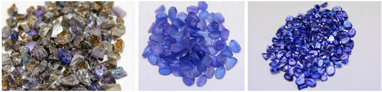
Figure 13. From untreated rough in sizes under one gram (left) to preforms that have been heated (center) and precisely calibrated finished stones (right), AG Gems must accurately estimate the final appearance and weight at each stage. Photos by Andrew Lucas, courtesy of AG Gems.
