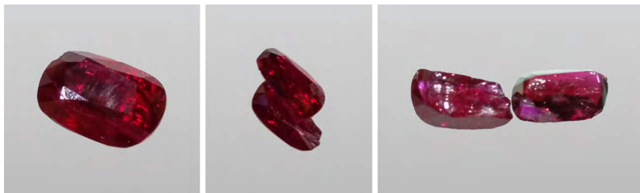
Figure 21. Left: The two pieces of a glass-filled ruby were combined to demonstrate its appearance before breaking. Center and right: The two pieces that broke during the setting process. Photos by Lai Tai-An Gem Lab.
