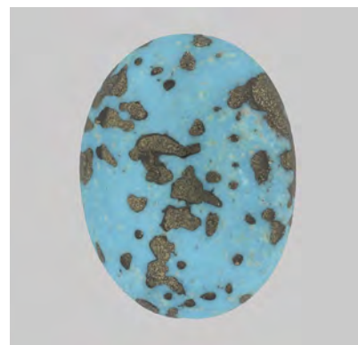
Figure 26. A 78.60 ct greenish blue turquoise oval bead with artificial metallic pyrite. The turquoise was filled with a mixture of crushed pyrite and polymer.
